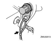
Secure the clamp bracket to the transom using the bolts provided with the outboard (if packed). For details, consult your Yamaha dealer.
